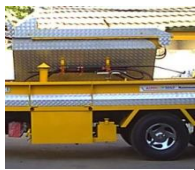
Hopper of asphalt mix
