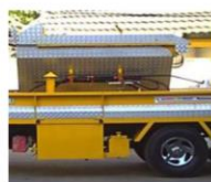
Hopper of asphalt mix
